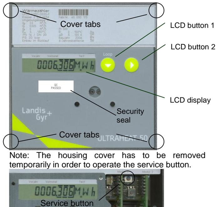
Note: The housing cover has to be removed temporarily in order to operate the service button.
