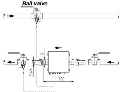
Example of mounting with a ball valve (recommended up to DN25)
