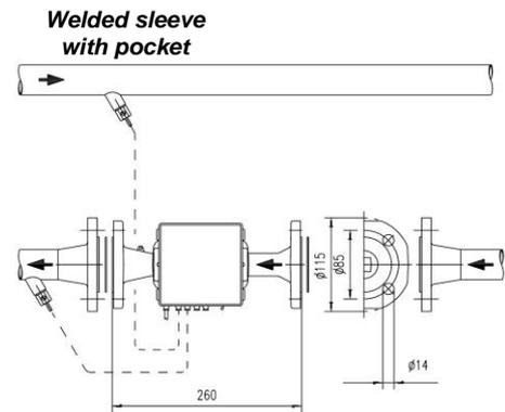
Example of mounting with pockets (recommended for > DN25)
