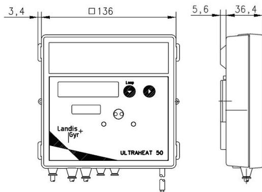
**For water temperatures below 10°C or above 90°C**, the electronic unit must be fixed on the wall (split mounting). For this purpose, remove the electronic unit from the adapter plate, unscrew the adapter plate from the volume measuring unit, and screw to the wall with plugs. Push the electronic unit on again.
